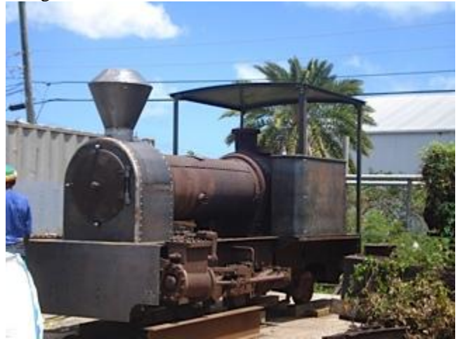
The "Marion" rebuilt with parts specifically manufactured in the UK. Next step is sand blasting, then painting and fitted with bits & pieces i.e. gauges & lights.
